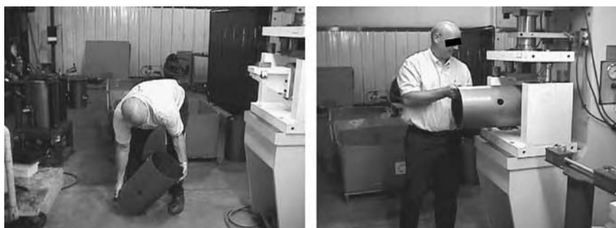
FIGURE 50.4 Lifting shell to press.
