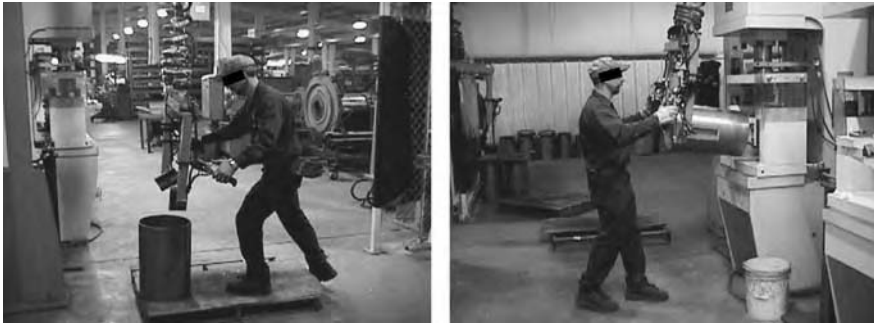
FIGURE 50.5 Using a manipulator to lift shell onto machine.
