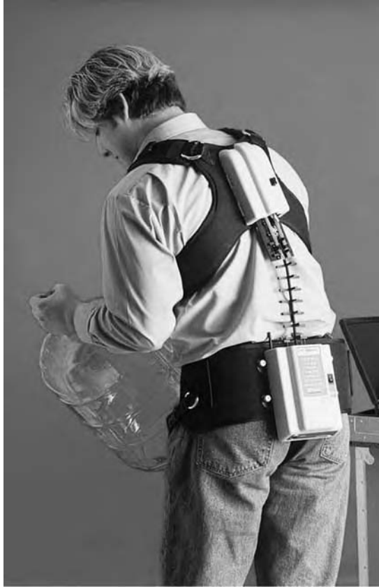
FIGURE 11.33 The lumbar motion monitor (LMM).
