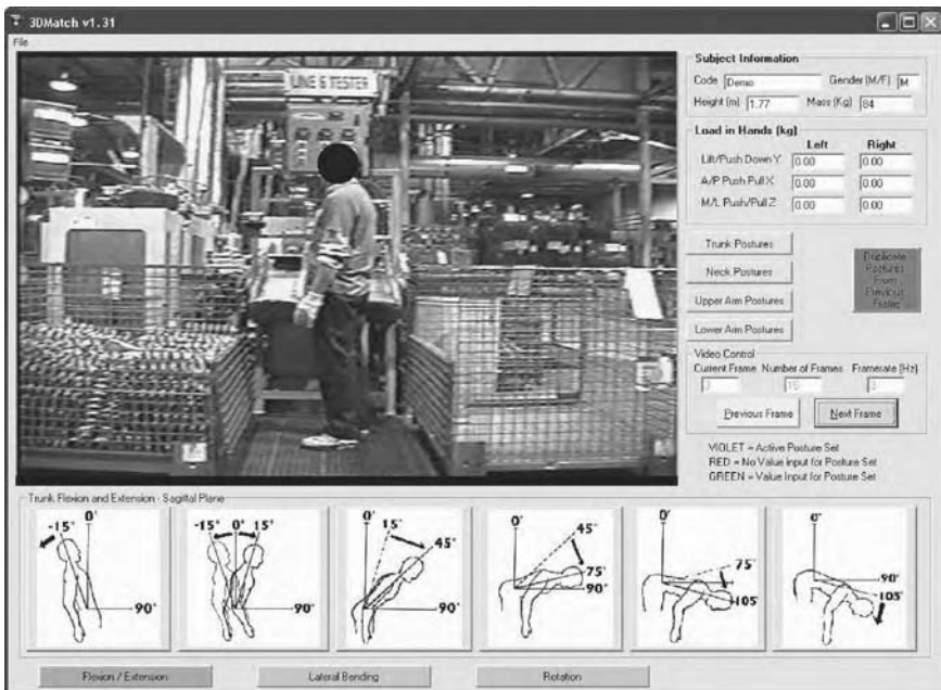
FIGURE 13.10 3DMatch user interface for using postural matching and external forces to calculate 3D spine loads using a biomechanical model.
